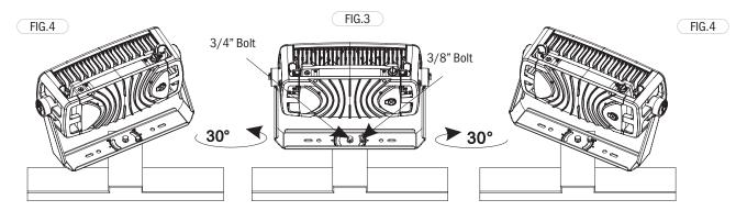
Use an hex wrench to loosen the adjustment screw. (Figure 5) Once the screw is loosened, adjust the angle of the fixture as needed. Retighten the bolts to secure the fixture in its new orientation. (Figure 6)
