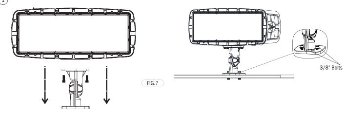
Adjust the lighting angle vertically, up or down, according to the required illumination needs. The fixture remains adjustable when hoisted or installed on a crossbar (Figure 8)
