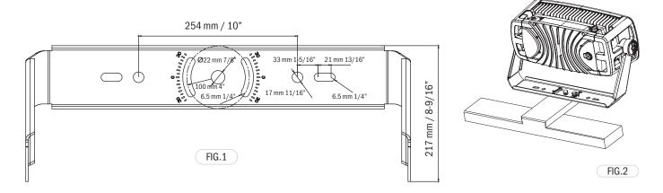
3 To set the left/right orientation, loosen the 3/4" and 3/8" bolts at the base of the Yoke Mount Bracket. Adjust the fixture to the required position. After positioning, retighten the bolts to secure the fixture in its new orientation.(Figure 4).
