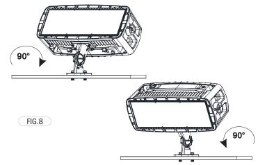
(3) Adjust the lighting angle horizontally to the left or right as needed to achieve optimal lighting coverage. (Figure 9)
